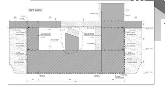
"Leftover" electrons are captured in a so-called beam dump. Here, 2000mm concrete alone cannot handle the requirement. Solid steel plates with a total thickness of 500mm complement the radiation protection. In total, approximately 300 tons of complementary steel was required locally at a beam dump.
