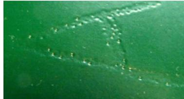
Surface contamination before galvanizing. This "A" was not visible after galvanizing, but after powder coating!
