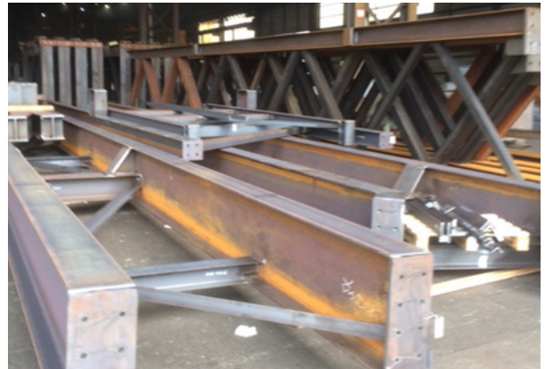
Large construction elements that are waiting for galvanizing. The lifting capacity at Galva Power is 12 tonnes.
