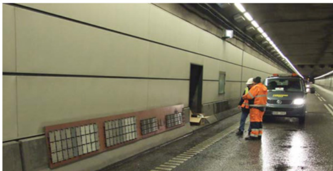
Steel samples placed close to the roadway in the Øresund tunnel. From an earlier research project with KIMAB.
