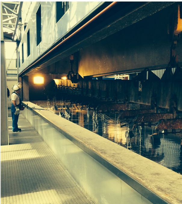
The big pot at Zinc Power Remels is entire 15.5 meters in length, 2 meters wide and 3.5 meters deep.
