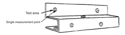
The requirement for "local coating thickness (minimum)" should not be compared to the results of individual measurements. The coating can be thinner or thicker at individual points, depending on the steel surface's composition and structure.
