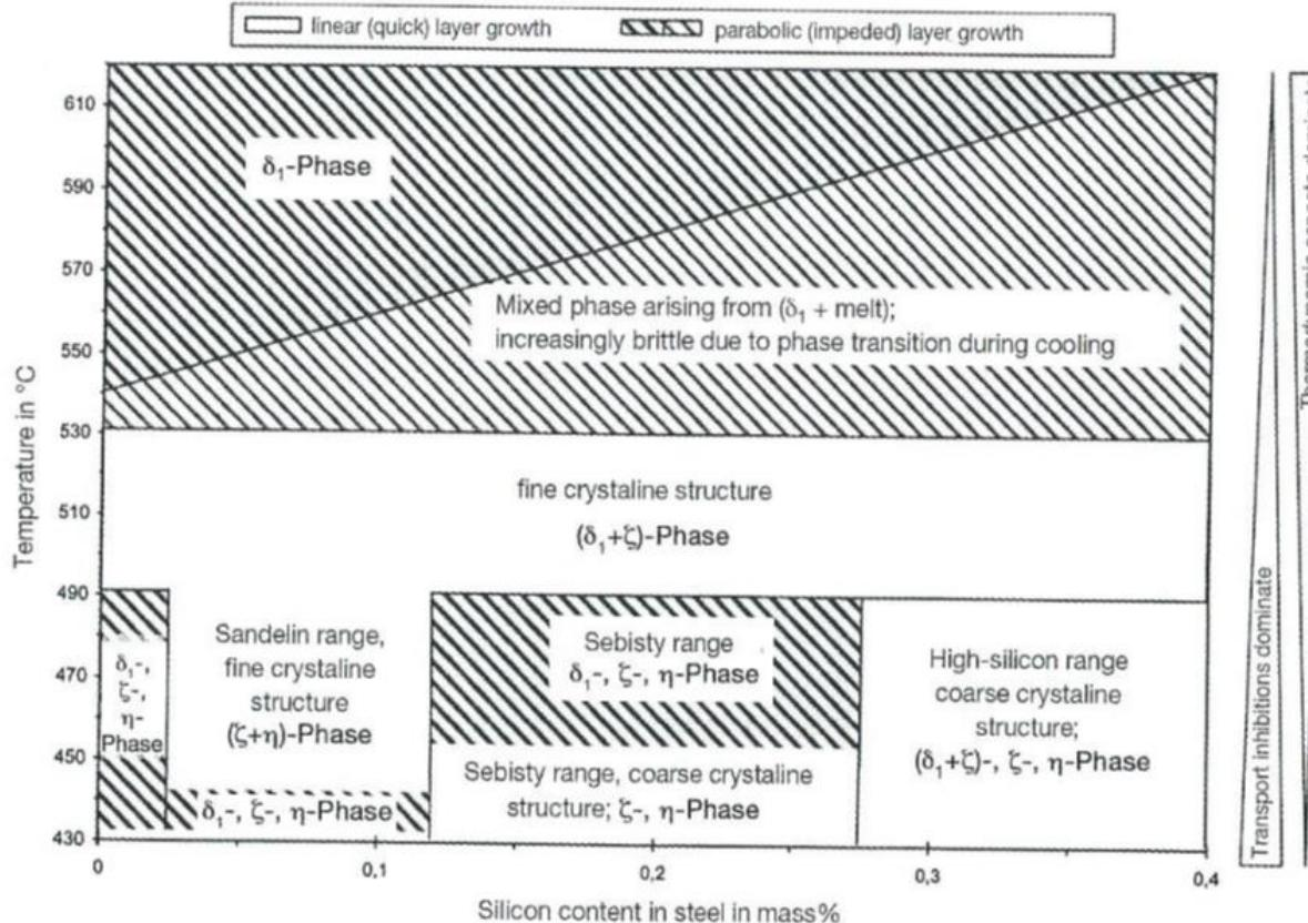
Fig. 40: General survey of the crystalline structure in hot-dip batch galvanizing for low-phosphorus structural steel in conventional zinc melt (galvanizing time > 5 minutes)
