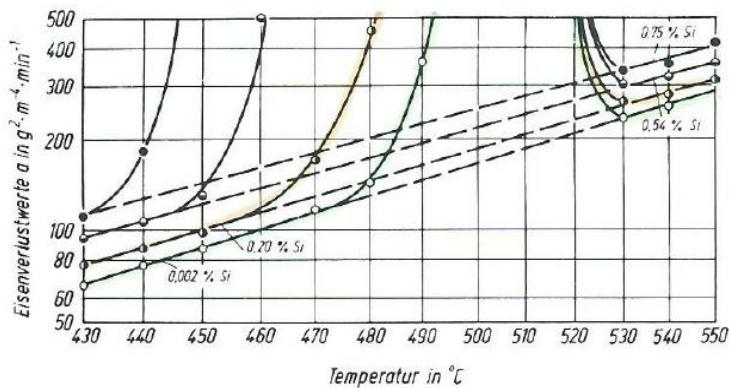
The Fe-loss for a 0,2% Si containing steel is only 15% higher than for a 0,02% Si containing steel!
