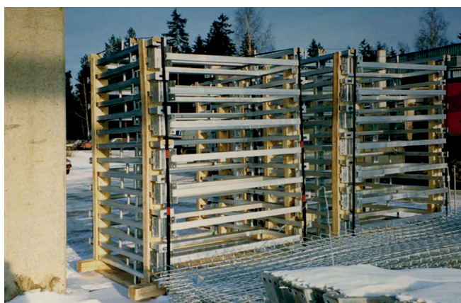
Figure 3. The galvanized steel should be stored with a slope and turned so that water accumulations are avoided. Spaces are placed so that no gaps occur and so that all surfaces are ventilated.
