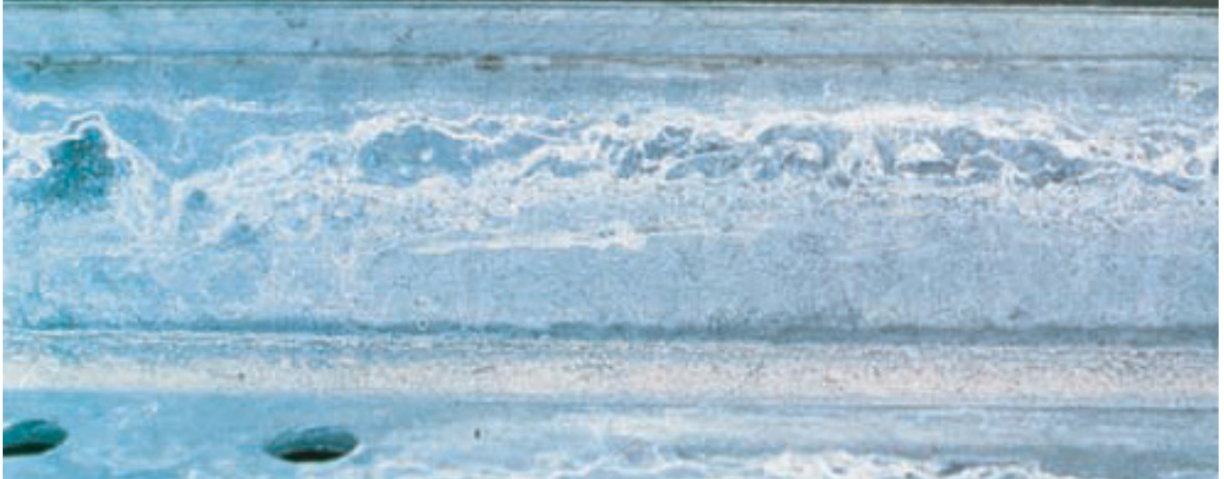
Figure 1. Wet-storage stain on closely joined angle irons after outdoor storage.
