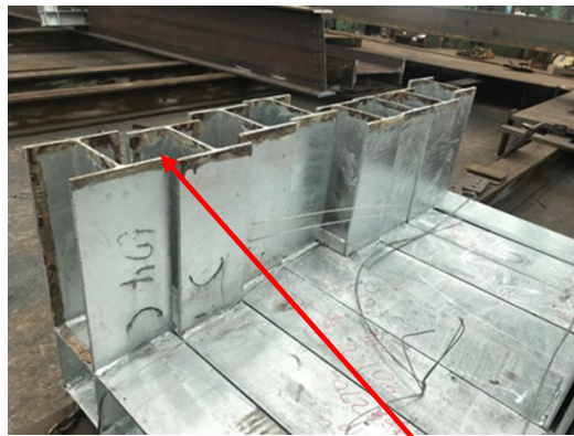
Uncoated areas with zinc to allow the weldability.
