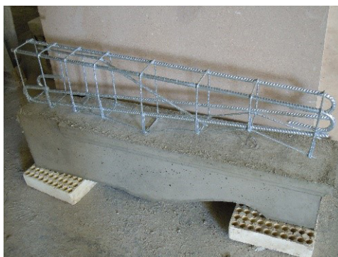
Hot dip galvanized steel reinforced concrete support beams for the balconies of an elegant apartment in Genoa. Galvanized steel reinforcement was chosen to best preserve the support beams of the balconies over time, in particular to protect them from smog, rain, frost and humidity. (Images courtesy of Prefabbricati Torti di Pietro e Lino Torti snc)
