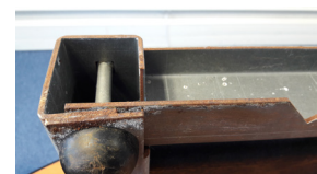
Figure 2. ZM steel with uncoated cutting edges where the self-healing effect has not been able to protect the surfaces.
